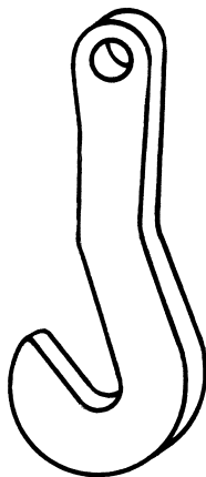
Fig. 10-1.1-15 Single Plate Hook
